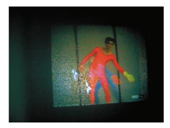
In this real-time human gesture recognition system, video images of a person are sent to a recognition module. The system does not require any sensors or cables to be attached to the subject's body. The key technology here is optical information processing. In the recognition module, video images taken by a CCD camera are presented to a holographic device that generates a vector representation of the gesture. The vector is then analyzed electronically to determine the gesture in real time.
